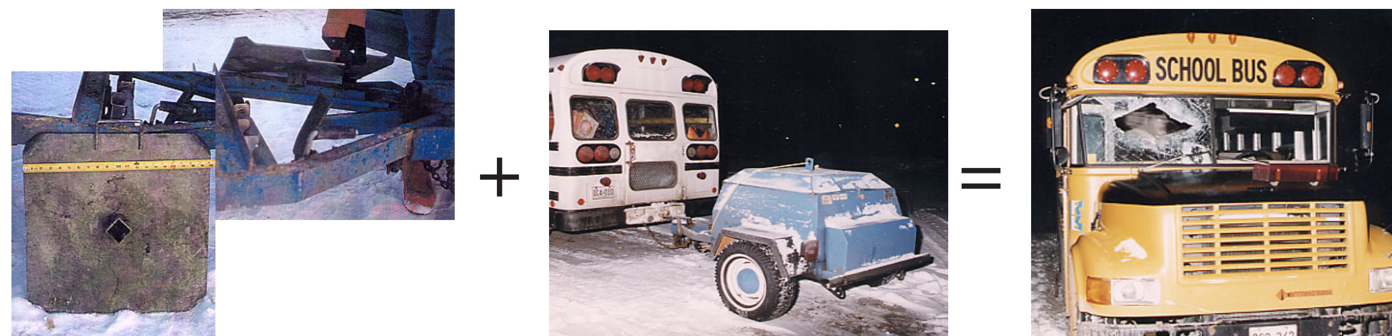
negligent worksite cleanup (sign base improperly placed)
